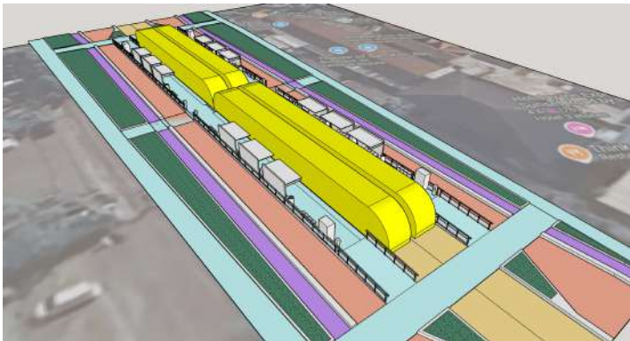
Figure 6. Example for two side platforms. © Authors. Source: Tools used: Google My Maps for Geographic positioning ; SketchUp for 3D layout of stations and platforms.
